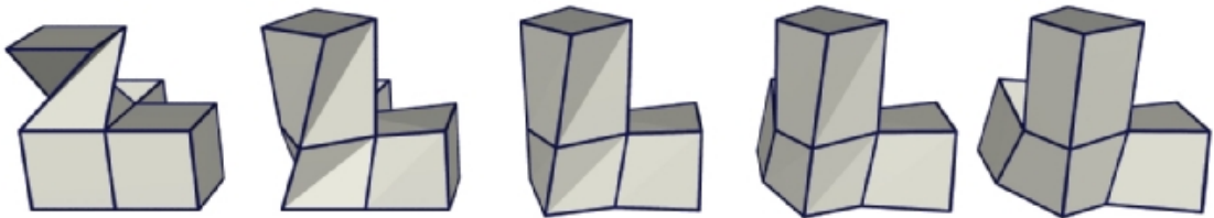
FIGURE 6.5: PQ perturbation without a closeness term applied to a highly un-planar mesh consisting of only a few quads.
